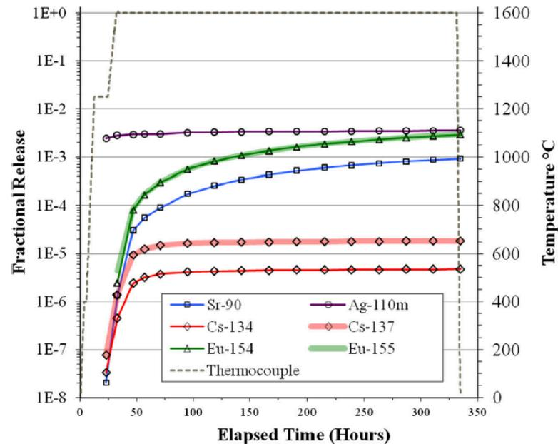
Compact 6-2-1, 1600°C 300 hour exposure showing fraction release of select fission products, reproduced from Ref. [1]
