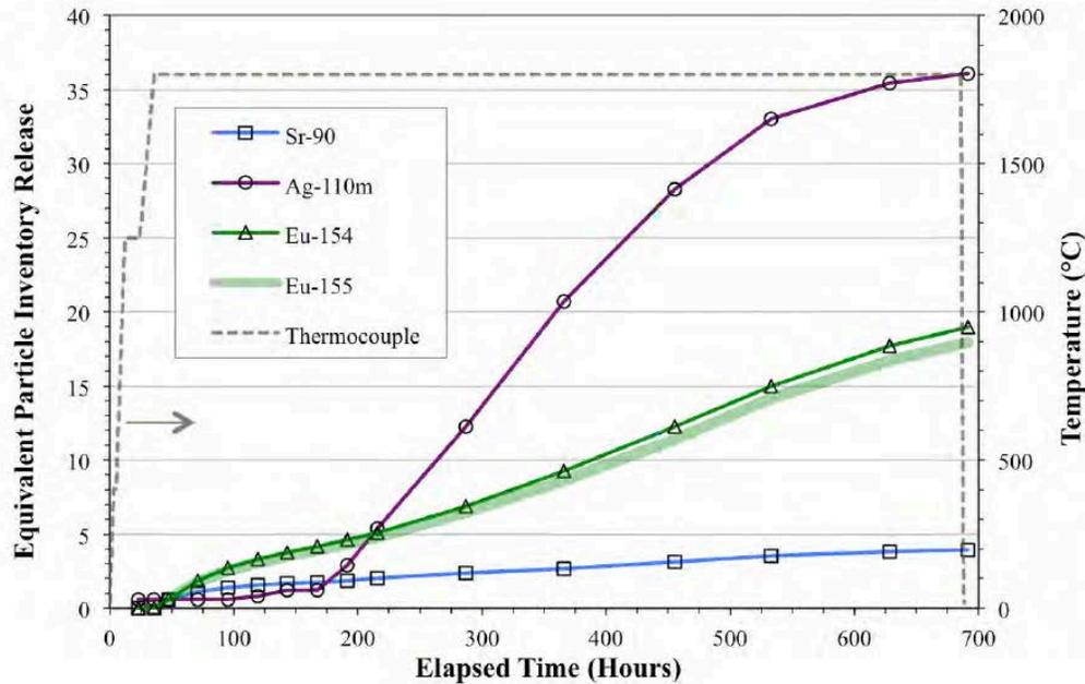
Cumulative release of silver, europium, and strontium, from Compact 4-4-2 loose particle testing, Reproduced from Hunn et al. (2016)<sup>[1]</sup>
