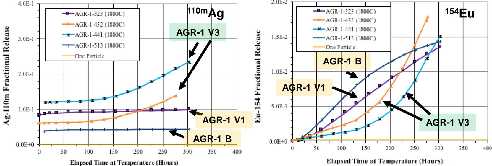
Fractional release measurements of  $^{110m}\text{Ag}$  and  $^{154}\text{Eu}$  from AGR-1 Compacts exposed to 1800°C for 300 hours, Compacts 4-4-1 and 4-3-2 were AGR-1 V3, while Compacts 3-2-3 and 5-1-3 were AGR-1 V1 and showed a difference in release behaviors. Reproduced from Morris et al. (2016)<sup>[1]</sup>
