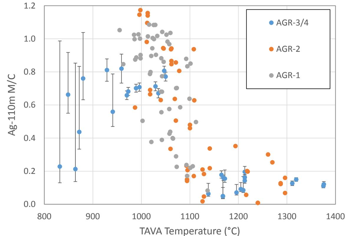
Inflection at 1096°C, Retained  $^{110m}\text{Ag}$  fraction as a function of time-average, volume average compact temperature, reproduced from Demkowicz (2017)<sup>[1]</sup>
