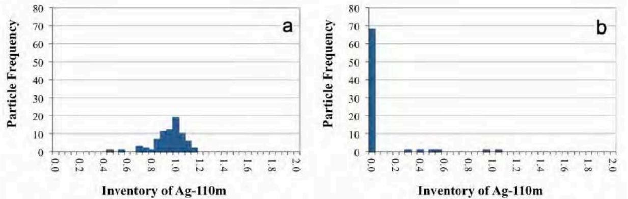
Ratio of measured  $^{110m}\text{Ag}$  versus calculated inventory for 75 particles from Compact 4-4-2 loose particle testing, a) as-irradiated and b) after 1800°C heating test, Reproduced from Hunn et al. (2016)<sup>[1]</sup>
