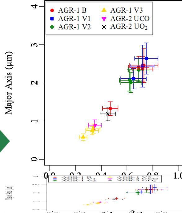
Average grain size (major, minor axis) for each constituent batch from AGR-1 and AGR-2, Reproduced from Gerczak et al. (2016)<sup>[2]</sup>
