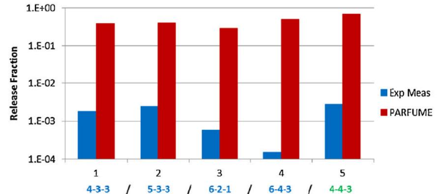
Fractional release data from safety tested compacts compared to predicted PARFUME release calculations, blue indicates 1600°C and green 1700°C, Figure reproduced from Collin et al. (2016) ref. [2]
