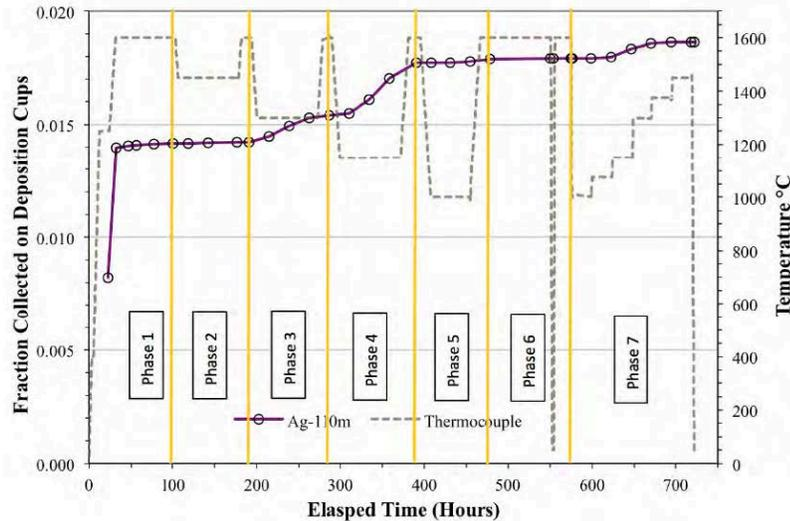
Fraction of collected of silver on deposition cups from Compact 4-2-2 thermal exposure test, varied collection efficiencies vary with temperature data does not directly scale with compact release fraction. Figure reproduced from ref. [1,2]
