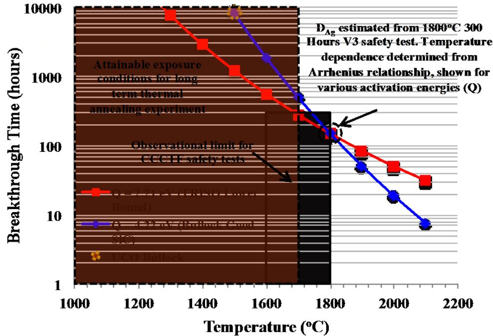
Estimated break-through time as a function of temperature based on 1800°C safety test results
