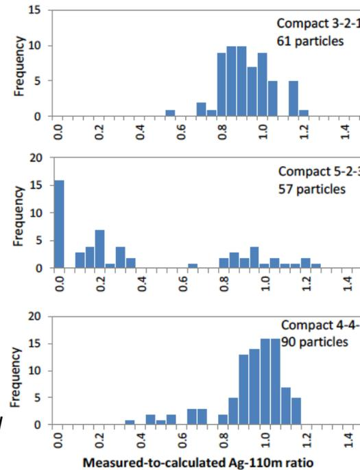
FP activity measured by gamma spectrometry, at ORNL the Irradiated Microsphere Gamma Analyzer (IMGA)
