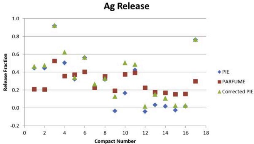
Compact release data (corrected from particle data) compared to predicted PARFUME release calculations, figure reproduced from Collin et al. (2015) ref. [1]
