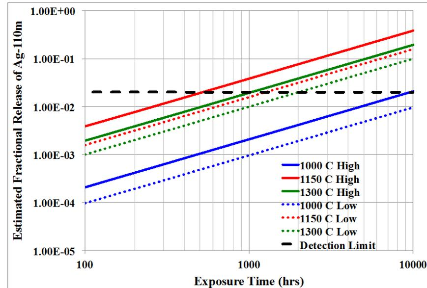
*Estimated avg. compact fractional release as a function of exposure time for the low temperature regime of interest, showing the high and low estimate from CCCTF testing of Compact 4-2-2.*
