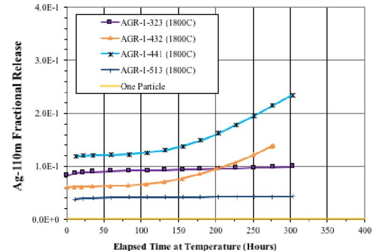
Fractional release measurements of  $^{110m}\text{Ag}$  from AGR-1 Compacts exposed to  $1800^\circ\text{C}$  for 300 hours, Reproduced from Morris et al. (2016)<sup>[3]</sup>
