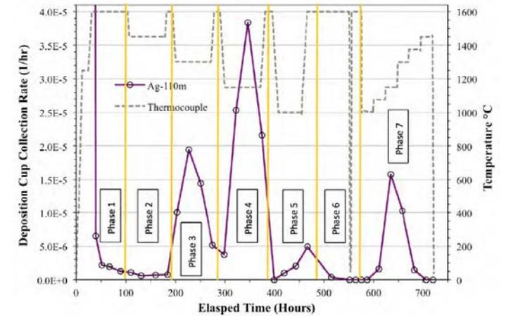
Collection rate of silver from Compact 4-2-2 thermal exposure test, Figure reproduced from ref. [1,2]
