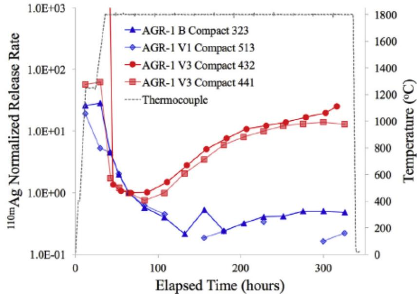
Normalized inventory release rates of  $^{110m}\text{Ag}$  from AGR-1 compacts exposed to  $1800^\circ\text{C}$ , Reproduced from Gerczak et al. (2016)<sup>[2]</sup>
